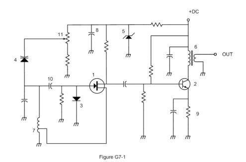
When designing or troubleshooting radios, amateur radio operators use schematic diagrams to describe circuits. Various symbols represent the different types of components. A typical schematic is shown in Figure G7-1.
